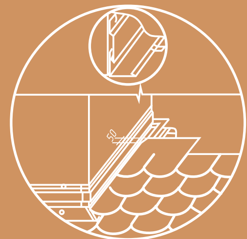
Variant 1 Abutments to the pipes (walls)
